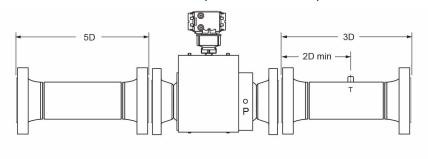
Figure 14: Piping Recommendation for Gas Ultrasonic Meter with a Flow Conditioner (optional)
