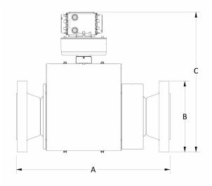
Figure 10: Dimension Key for DN400 and larger (16-in and larger) Meters with Dual Transducer Shrouds (See Table 17 and Table 18)
