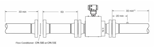
$3D \min^{(1)}$  = Additional pipe length may be required for additional taps (i.e. sample probe, test well, etc.).
